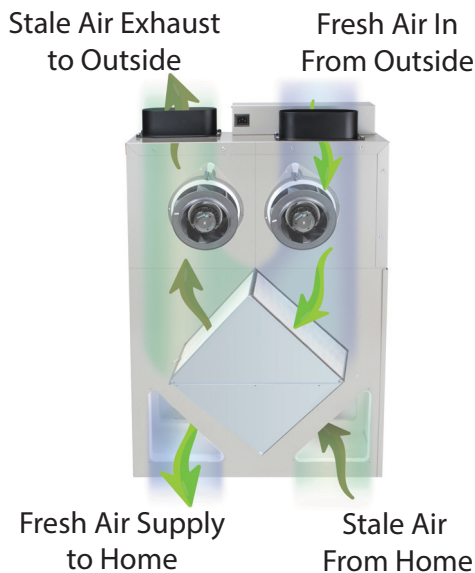
Fig. 4 - Airflow During Air Exchange
